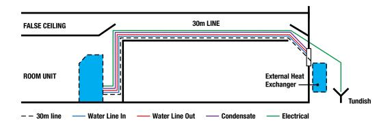
By joining 6 flexible line of 5m, it is possible to install the external heat exchanger more than 25 metres from the area cooled by the room unit. The lines may run in a false ceiling, false floor or along a carpet. The flexible line will pass through a hole in the wall or ceiling of 5cm x 8cm if required. The external heat exchanger is supplied with hanging chains.
